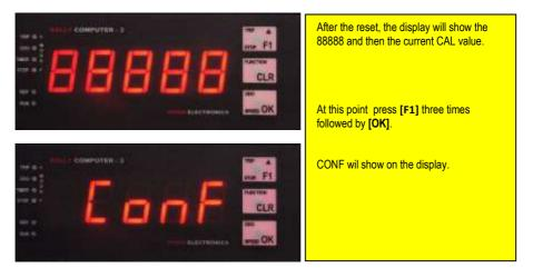
To select a function press **[F1]** and confirm with **[OK]**. To change the value press **[F1]** and we confirm by pressing **[OK]**. The change will be confirmed by a quick display blink. To exit press **[CLR]**.
