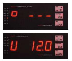
[TRACK] – course – When using GPS, it shows the route course. The display shows the degree symbol on the left, and the current value on the right which is the deviation angle from the North.
