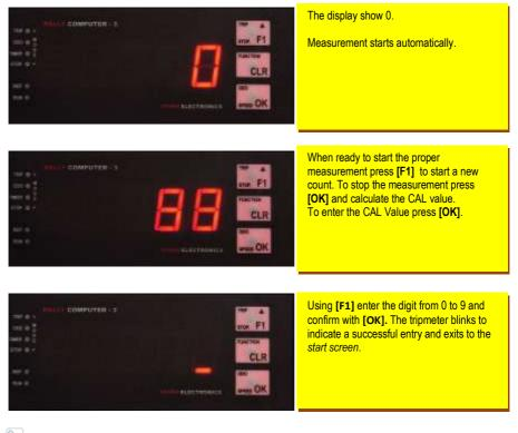
Muto-calibration using inbuilt GPS module.
