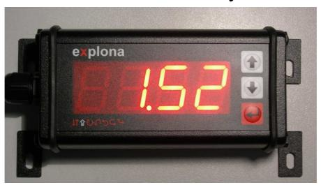
**explona repeater/mini** is the smallest device of **explona** family. It was designed mainly as an additional display for a driver. It can show data supplied by main odometer (e.g. **explona dakar**).
